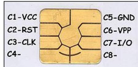
Gambar 5 Smart Card's pin contact
